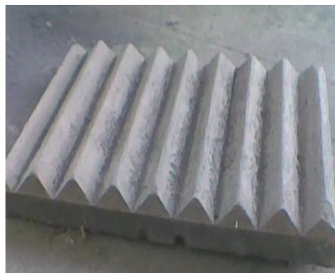
Figure 23: A fixed jaw is often used in the quarry industry.
