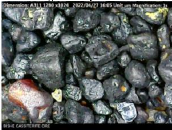
Plate 4.5: Micrograph of Bishe Cassiterite ore Sample under plane polarized light (X 1000)
