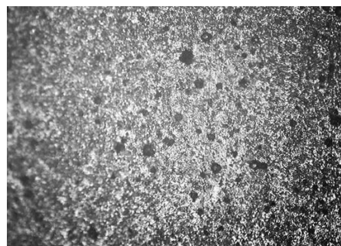
Plate 1a: Microstructures of as-cast ductile iron, ×100.
