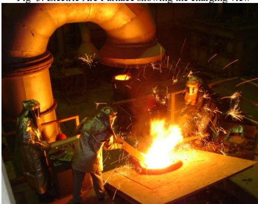
Fig 7 the de slagging process in the Induction furnace
