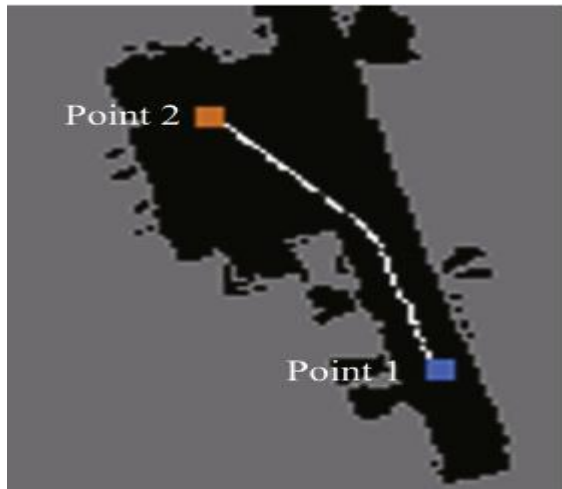
Figure3: Map of the floor in the hospital and path produced by the path planning method
