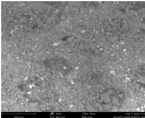
Plate 4.1: SEM Result of Bishe Cassiterite Sample (x 500)
