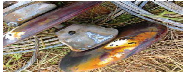
Fig. 1. 3: Damaged glaze on porcelain insulator due to power arc from lightning.
