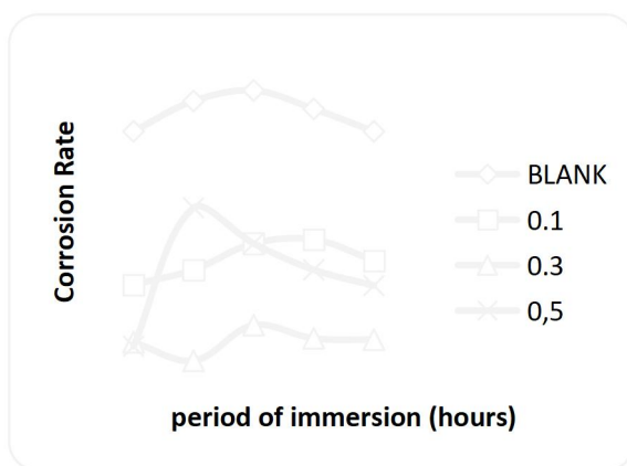
Fig. 3.3: Corrosion rate, C_R as a function of time for mild steel in 1.5M HCl in the absence/presence of MI extracts (leaf)
