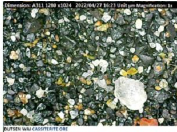
Plate 4.6: Micrograph of Dutsenwai Cassiterite ore Sample under plane polarized light (X 1000)
