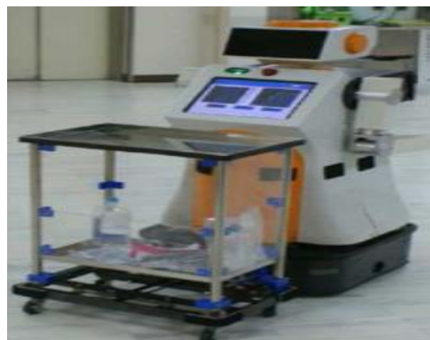
Fig. 2. Traction type autonomous omni-directional mobile robots.
