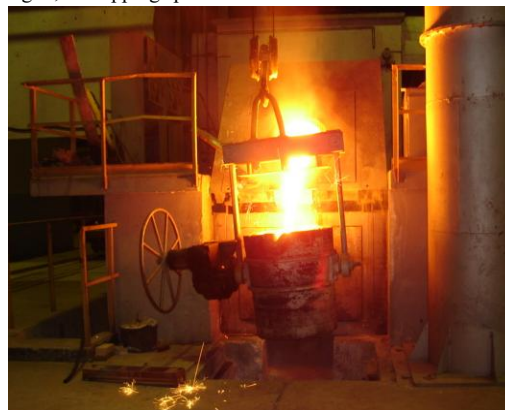
Fig 8: the teeming process from the induction furnace
